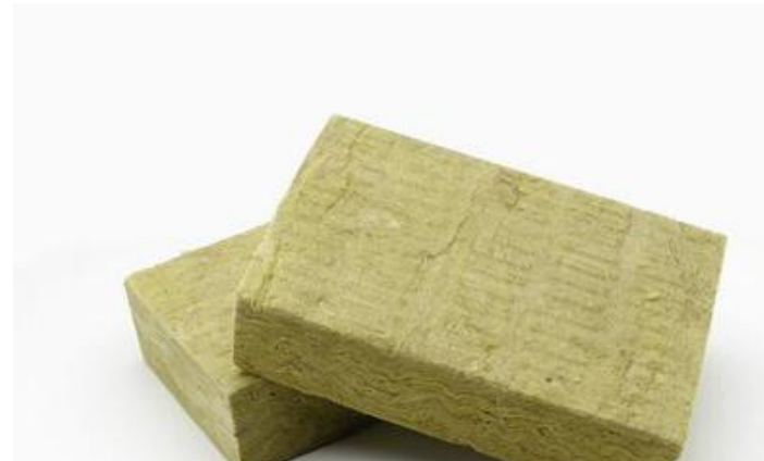
Rock Wool Insulation 100mm thickness U value 0.35-0.44 W/m 2 K
