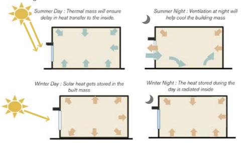
Figure 6: Use of thermal mass and solar gains to make indoors comfortable
