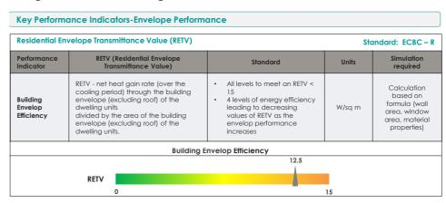
**Figure 16**: **Envelope Performance indicator -** Residential Envelope Transmittance Value (RETV)
