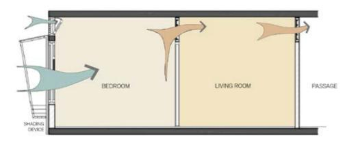
Figure 5 : Ensuring cross ventilation through living spaces
