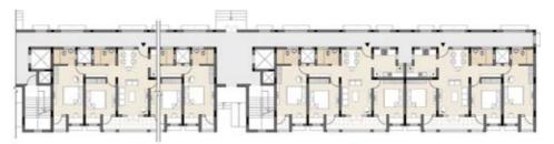
**Figure 38 :** Compact planning keeps exposed wall surfaces to a minimum and reduces heat loss from the building.
