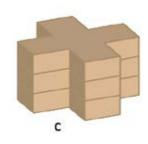
**Figure 3 : Compactness of Building -** Compactness depends on the geometry of the building and it varies with the building typology. In this figure the surface to volume ratio increases from A to C as the built form gets more complicated, the compactness reduces.
