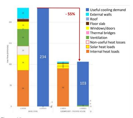
**Figure 35 :** Sensible cooling demand reduction for row house (1.2B) in Bhubaneswar (Warm & Humid Climate)
