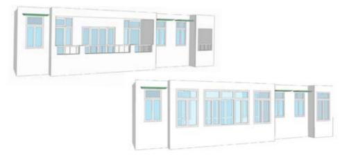
**Figure 39 :** A south facing glass enclosed balcony in cold climates can catch the winter sun and help warm the external walls and insulate them for the night.
