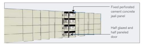
**Figure 11:** Shading devices and screens are modeled as per design to get accurate daylight and EPI results
