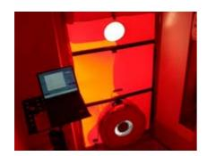
Figure 28: Airtightness test [Source PHI]
