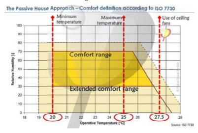
**Figure 24 :** The Passive House standard uses a comfort definition according to ISO 7730 [Source ISO 7730].
