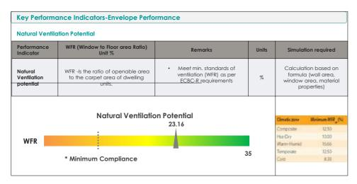
Figure 17: Envelope Performance indicator - Window to Floor Area Ratio.
