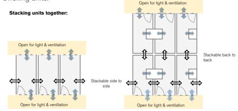
**Figure 39 :** Introducing courts for internal ventilation allows stacking units back to back. This gives **greater economy** of construction as **shared walls increase** and **street frequency decreases.**
