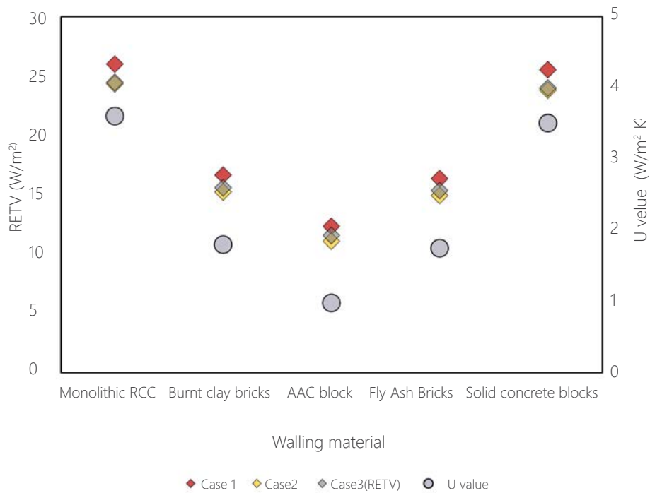
Figure 144: U-value and RETV for walling materials
